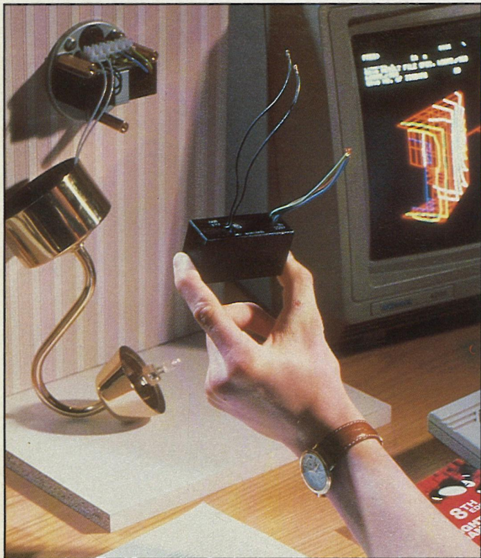
Figure 3. Line regulation is one of the safety features incorporated into this GTE electronic transformer.
